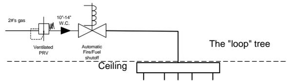
In summary, your gas distribution system should be designed to accommodate simultaneous peak flow conditions, with a bit of “headroom” in reserve. Don’t be too quick to blame equipment for problems in operation, especially if the problem is intermittent. Challenge the design professionals engineering your space to provide systems that are scaleable and sensible given your immediate and future energy needs.
